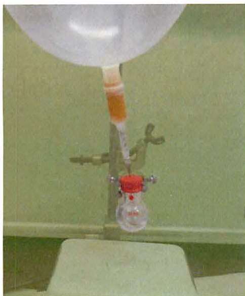
Figure 1. The reaction mixture after purging with hydrogen.
