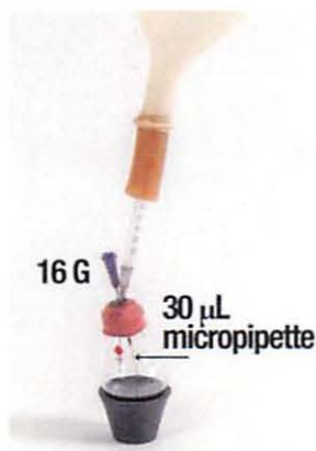
Figure 4. The use of a 30 \mu\text{L} micropipette and a 16G needle to sample the reaction by TLC.
