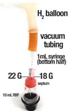
Figure 5. Purging of 10 mL RBF with \text{N}_2 followed by \text{H}_2 .
