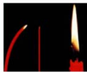
When the tip alone is illuminated bending still occurs
